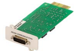
BD relay card (для ИБП Eaton 9130)
